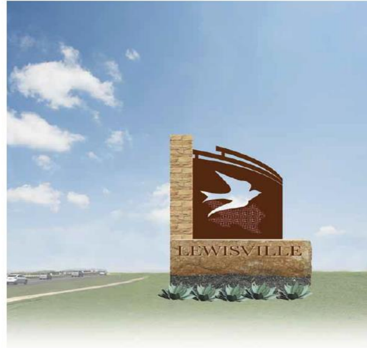
Scale: Stacked Stone Column 8 ft tall / 7 ft wide slab base / 1 ft tall lewisville letters
