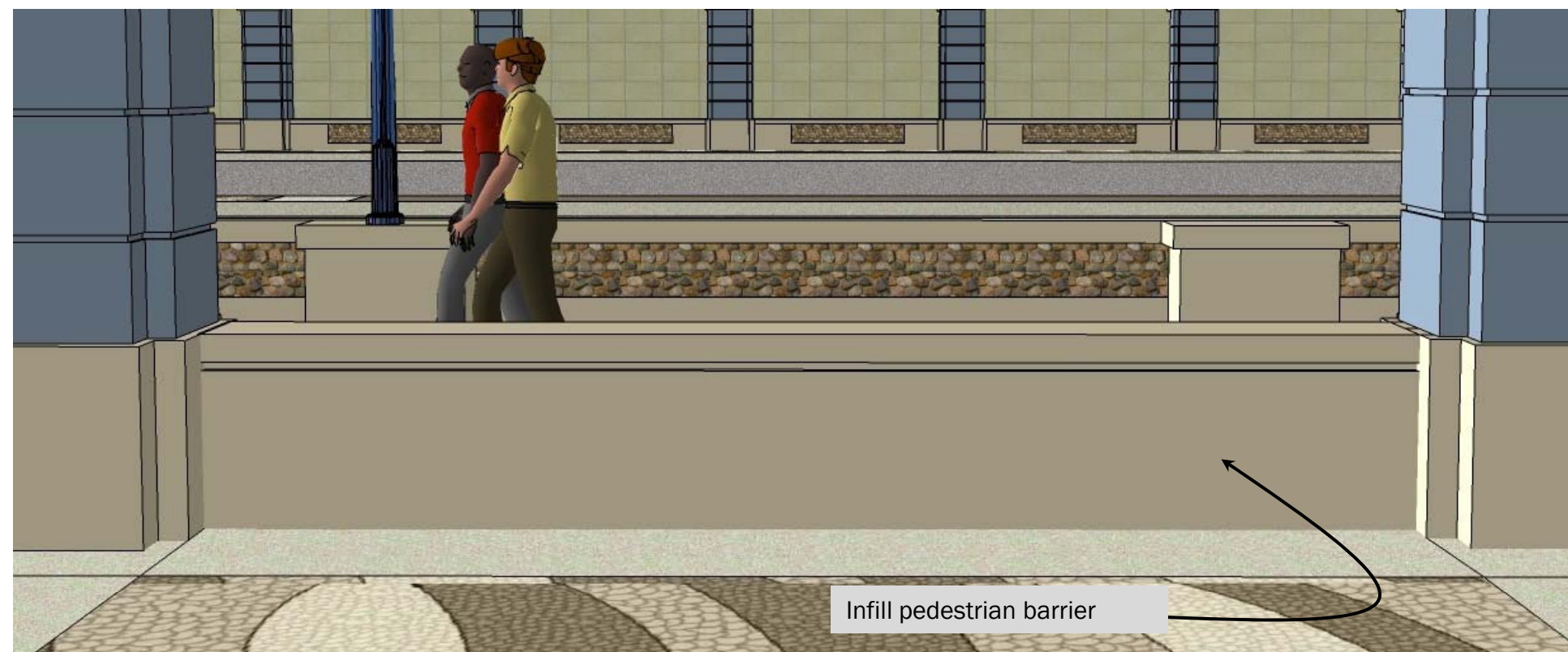
View of infill barrier between column lines to match base treatment on bridge columns – Cross-street view
