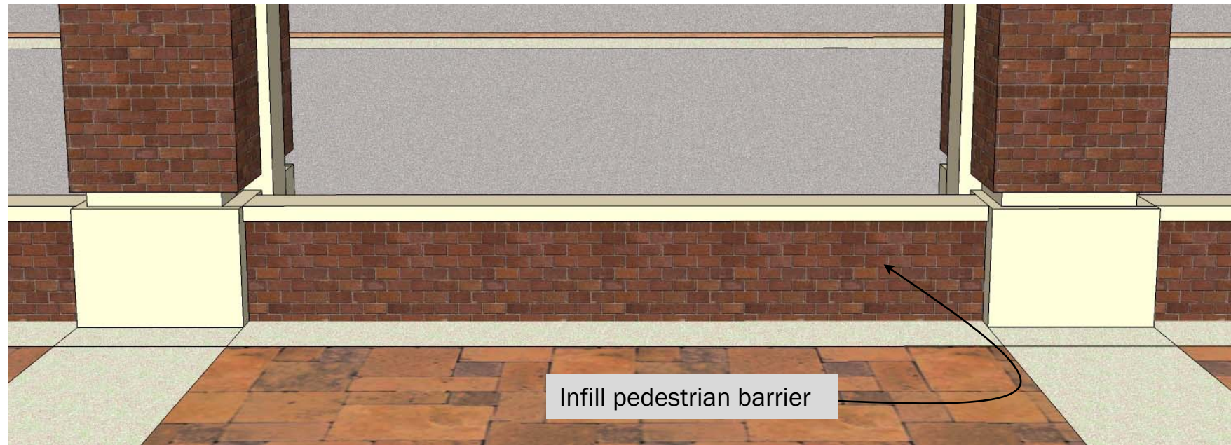
View of infill walls between column lines - brick texture and color - Walkway view
